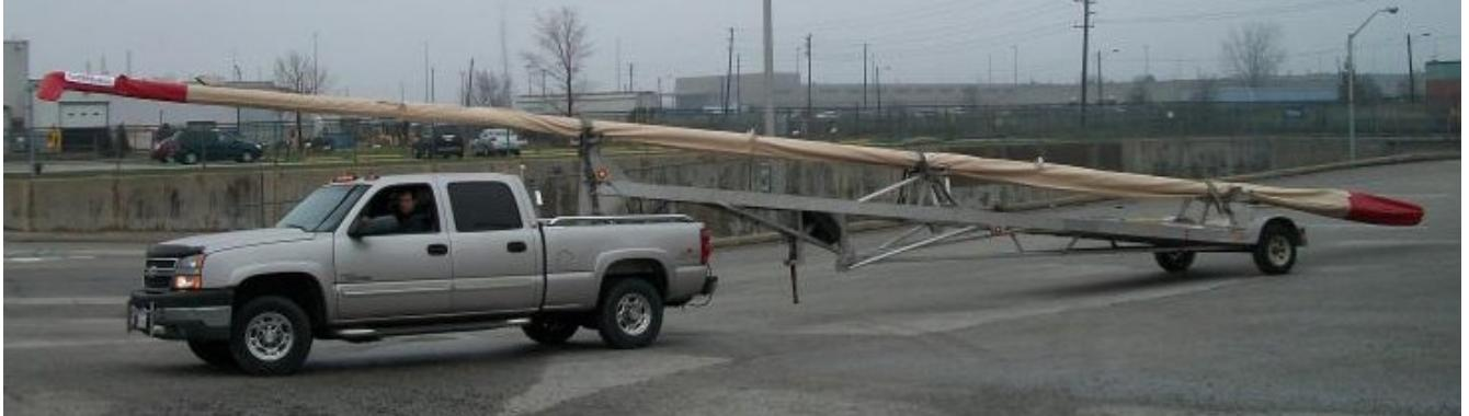
or, it could be an inexpensive utility or 2<sup>nd</sup>-hand trailer bought near the mast's location and then modified to add a support fork and lights.
