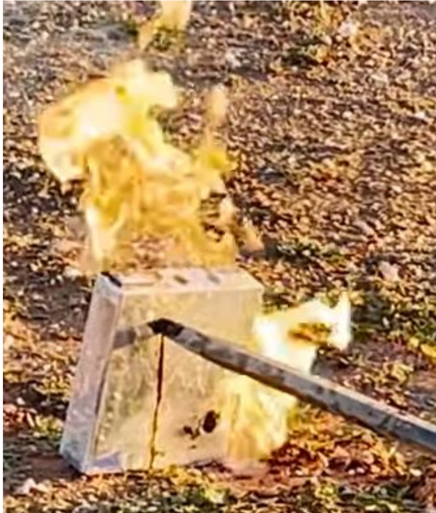
https://www.youtube.com/watch?v=07BS6QY3wl8 Physically puncturing LiFePO4 Battery
